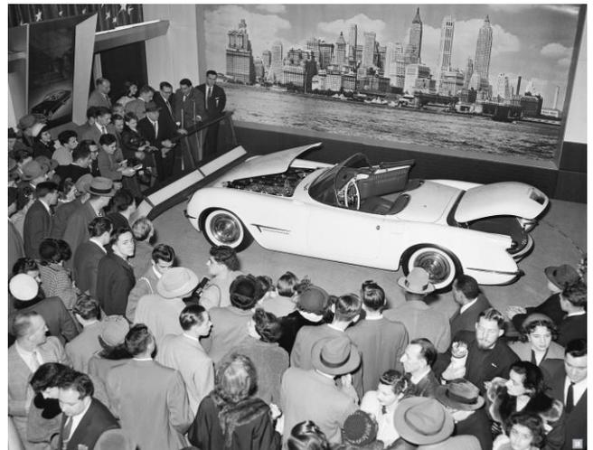
Manufacturing problems such as Glass Reinforced Plastic (fiberglass) molding techniques were far from being perfected and additional experimentation was necessary before company heads were convinced that fiberglass was the way to go and production could begin. Techniques evolved during the first production cycle and, as a result, each 1953 Corvette is slightly different.
