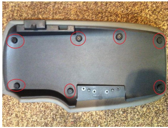
The 7 T-15 Torx Screws to remove bottom plate
